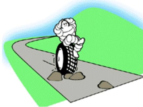
Tyres absorb the shocks due to obstacles and cushion the vehicle from other irregularities in the road, ensuring driver and passenger comfort as well as contributing to the lifestyle of the vehicle.
