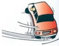
Numerous tests have shown that it is easier to control the front wheels than those at the rear. Front tyres generally wear quicker than those fitted at the rear, particularly on front wheel drive cars, which are currently in the majority
