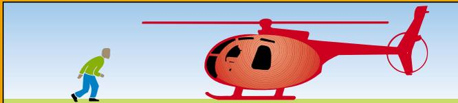
Do not approach or leave without the pilot's visual knowledge. Keep in pilot's field of vision at all times. Observe Helicopter Safety Zones (see diagram right)
