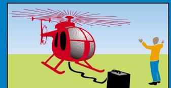
After hooking up cargo sling, move forward and to the side to signal pilot. Ensure sling is not across skid. Never ride on sling.
