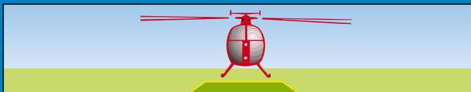
Keep helipad clear of loose articles – water-bags, ground-sheets, tins, etc. Secure other gear from effects of rotor wash.
