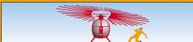
Do not approach or leave a helicopter when the engine and rotors are running down or starting up.
