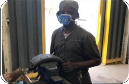
Use a mask or a respirator to prevent dust and asbestos inhalation while working on brake pads and other spare parts. Avoid exposure to asbestos dust, it is highly toxic.
