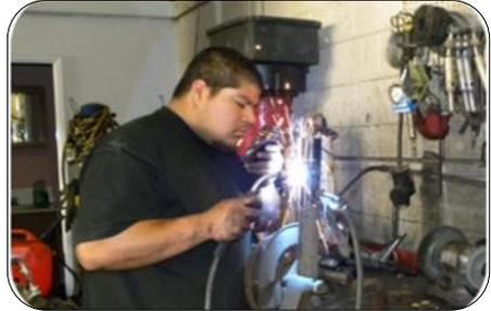
Do not weld without the proper equipment. Welding fumes are toxic and long-term exposure to the welding arc damages eyes.
