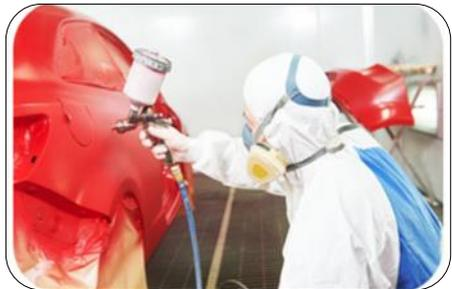
Use PVC gloves, safety boots, protective overalls with hood and an air-purifying respirator when painting. Avoid exposure to toxic fumes.
