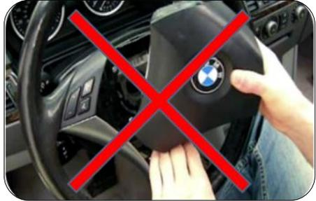
Never place your head or body close to the front of an undeployed airbag, especially when fitting it, or removing it from a vehicle. Never hold the trim cover facing towards you.
