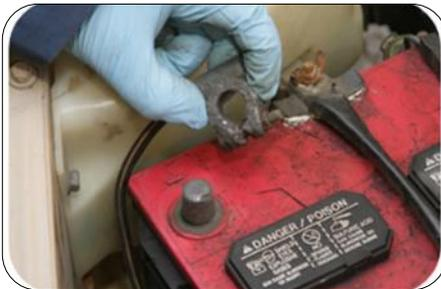
Use safety gloves, boots and goggles when changing/refilling battery acid and cleaning terminals. Acid is corrosive and can cause burns to skin and eyes.
