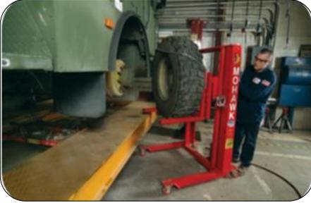
Use the right tools and equipment when performing operations such as handling heavy-duty tyres or transporting large fuel drums, to reduce the risk of workplace accidents.
