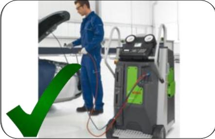
Use appropriate tools and personal protective equipment (safety boots, goggles, gloves) when loading refrigerant gas.
