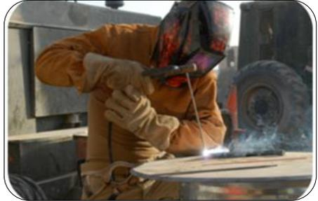
Use an appropriate full face mask, safety boots, gloves and overalls when welding. Protect yourself from fire risk and your eyes from the welding arc.
