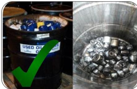
Drain oil from filters into a container and store the filters in a labelled drum, on a hard surface. Filters should be disposed of by a licensed contractor.
