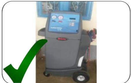
Whenever possible, prioritize refrigerant recovery using appropriate equipment, rather than venting gas into the atmosphere. Ensure proper disposal/exchange of empty cylinders by authorized contractors.
