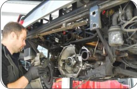
Do not handle brake pads, clutch parts, or gaskets without protective equipment, as they may contain asbestos. It is not possible to distinguish if a component contains asbestos just by looking at it.
