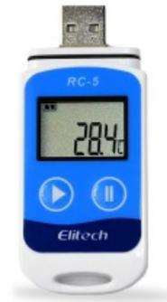
Once activated, temperature dataloggers can be dropped into a box or package of health items and retrieved on the other end. Temperature dataloggers can therefore be used when shipping single boxes, or when shipping pallets or large volumes of items, and can be used when shipping across multiple carriers or multiple modes of transportation.
