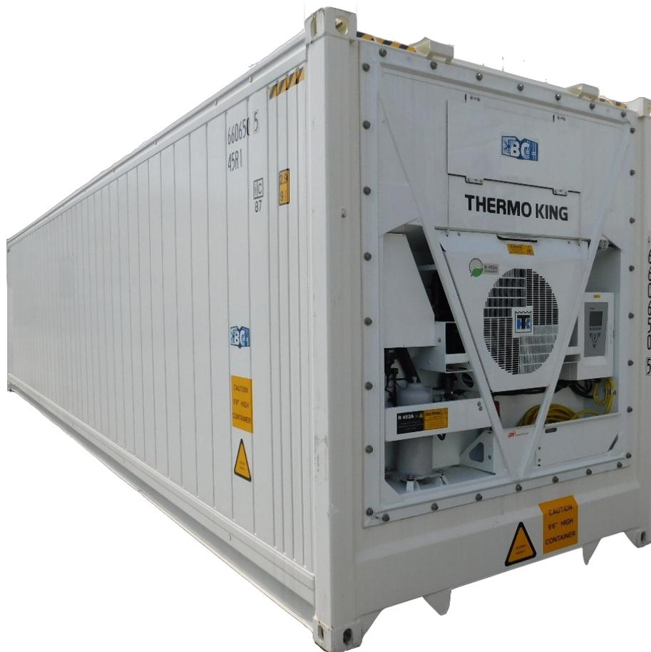
All reefer containers used for sea shipping must undergo what is known as a pre-trip inspection (PTI). Unless the reefer container is owned by the sender of the cargo, PTIs are undertaken by the shipping company. PTIs validate the condition of the container, the refrigeration equipment, and the monitoring equipment, and are rated for 30 to 120 days, depending on the needs of the shipping line and policies of the company.
