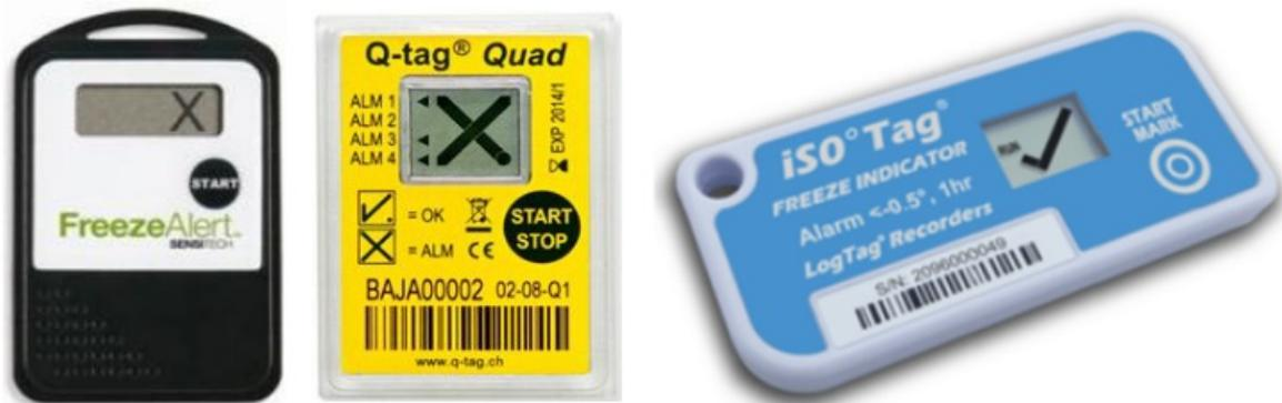
**Electronic Shipping Indicators** - more sophisticated devices that show if a product has been exposed to temperatures beyond the assigned alarm settings. They record the temperature at regular intervals during a certain period (normally not exceeding 20 days due to memory overflow). They have a digital display that reflects if the item being shipped crossed the alarm thresholds.
