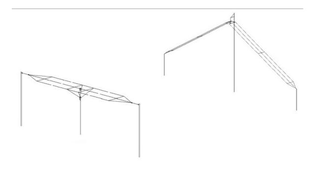
**Horizontal Configuration** – The di-polar antenna is tautly suspended from both ends at equal heights. The cable connection to the base station is free hanging, though ideally it will still be secured to something near the ground level or anchored to a sturdy pole to prevent movement in the wind, and to take weight off the installation. The horizontal configuration is considered the best case, and will carry a signal the furthers.
