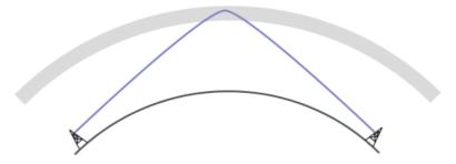
While HF may offer an advantage in the distance of its communication, it also comes with limitations. Notably, the equipment required to transmit and receive HF signals is bulky and large, and requires a significantly larger antenna and a larger energy source. Generally speaking, there are no good solutions for handheld mobile HF radios used by humanitarian agencies – HF is almost always limited to vehicles and stationary buildings.
