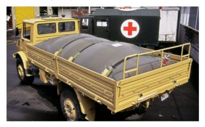
Fuel bladders on a vehicle should be properly braced and secured, just like any other load. Tie downs need to accommodate the full weight of the fuel, and the bladder itself should be properly rated for use as mobile transport. Consult with the manufacturer before using a bladder for transport purposes.
