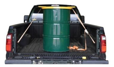
Full drums should ideally be transported upright, along their flat edge to avoid rolling around while in transit. Avoid double stacking full drums unless there is specialized railing or securing mechanisms in place.
