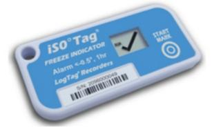
**Electronic Shipping Indicators** - more sophisticated devices that show if a product has been exposed to temperatures beyond the assigned alarm settings. They record the temperature at regular intervals during a certain period (normally not exceeding 20 days due to memory overflow). They have a digital display that reflects if the item being shipped crossed the alarm thresholds.
