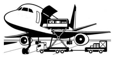
K-loader - Cargo requiring high lift loading alongside an aircraft
