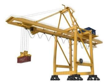
**Gantry Crane** - Another form of movable container crane, one that specifically straddles both side of a vessel or stack. Gantry cranes can be large enough to reach over the deck of an entire vessel, but may also be used for loading and offloading trucks or piles of cargo.
